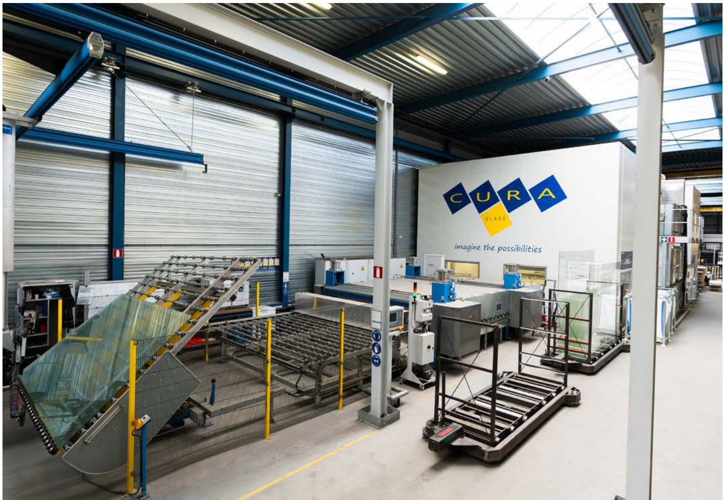
Our laminating line for the production of CURA Safe
