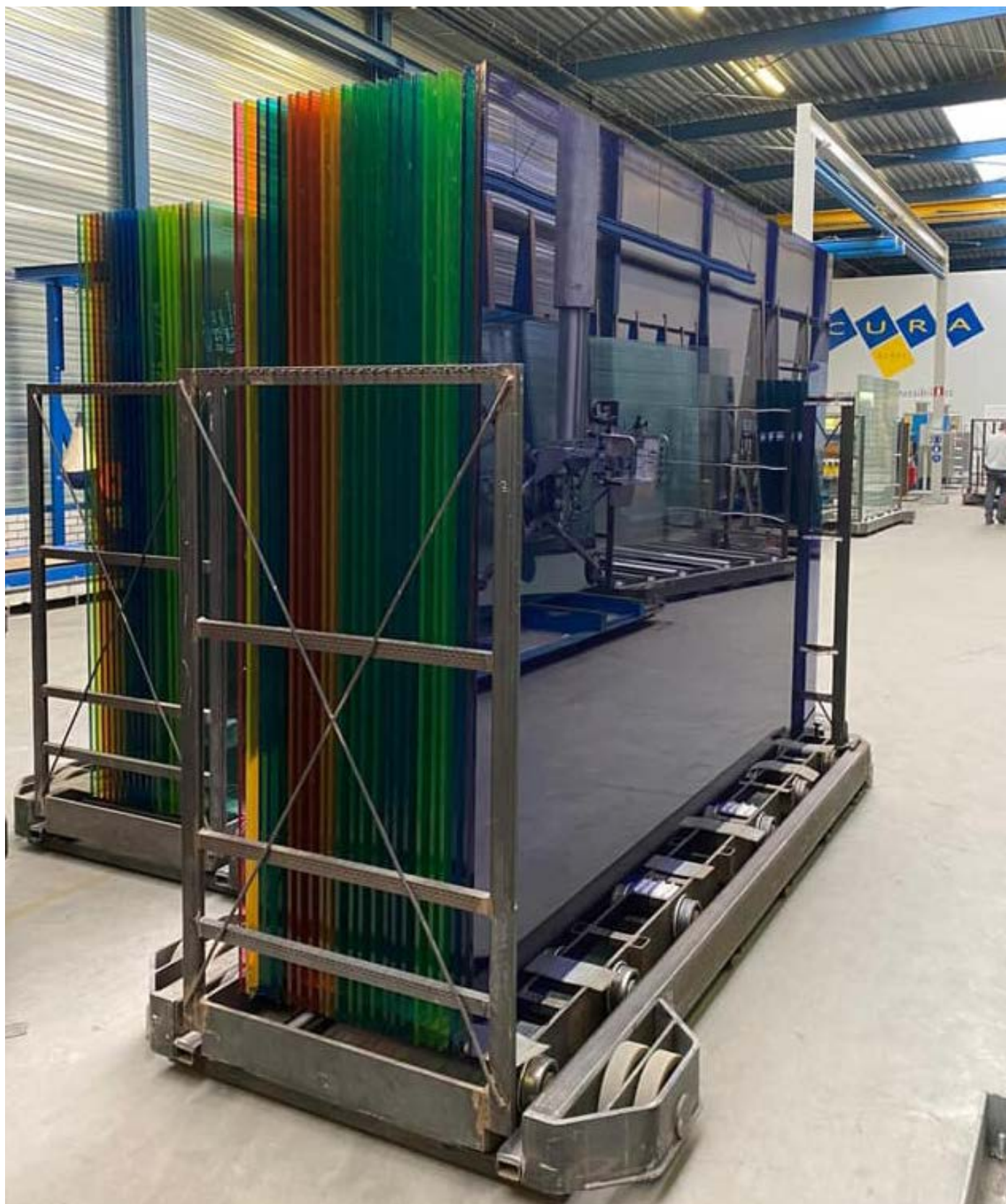
Clear laminated glass with Vanceva coloured interlayers
