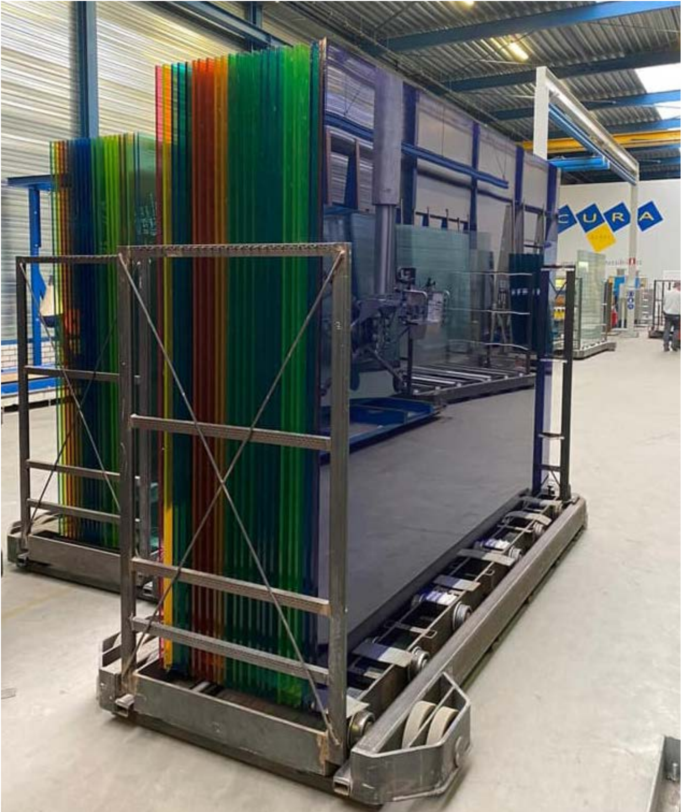
Clear laminated glass with Vanceva coloured interlayers
