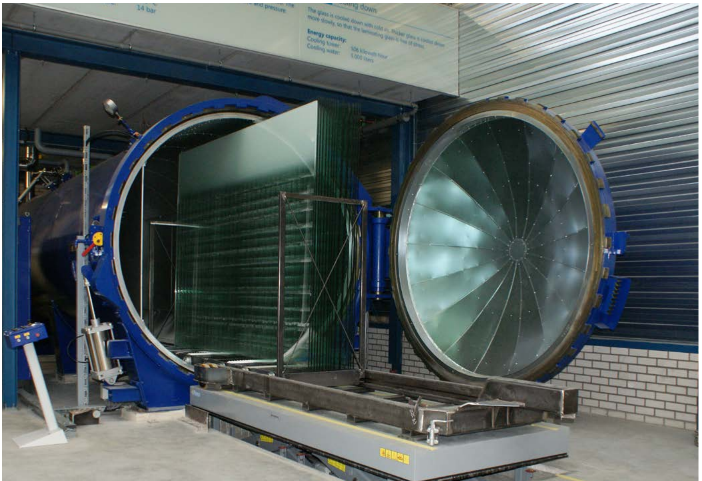
The autoclave is part of our production process of CURA Safe laminated glass with PVB-interlayer
